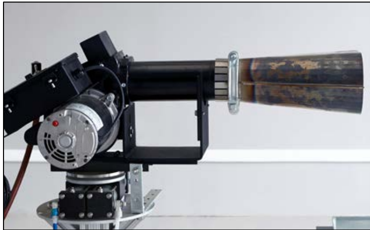
Figure 2. Carlin 200 CRD (Modified Gun-Type Oil Burner)
