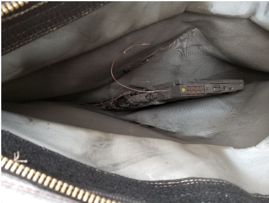
Figure 18. Containment Kit Post-test
