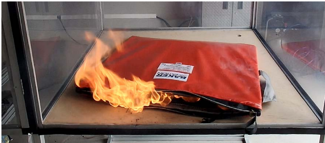
Figure 14, Initial Battery Ignition
