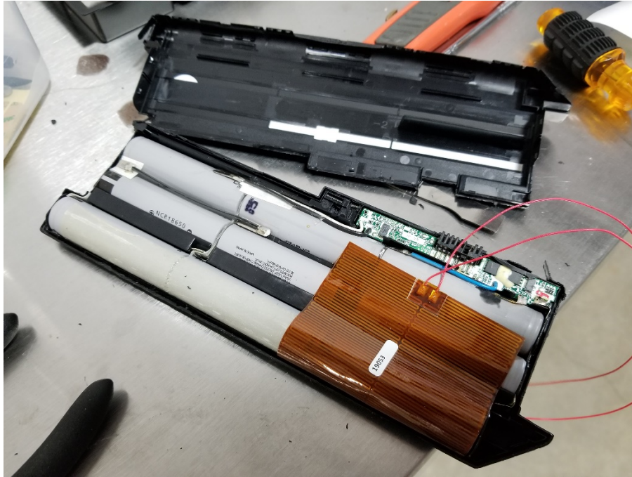
Figure 3. Film Heater on Cells
