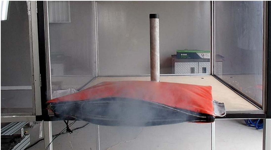
Figure 6, Initial Battery Ignition
