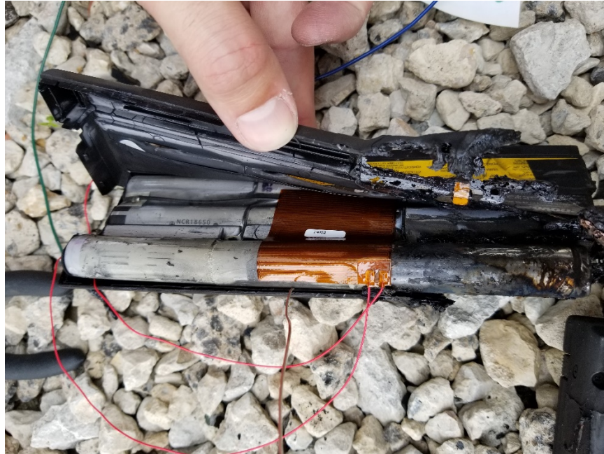
Figure 11. Film Heater on Cells
