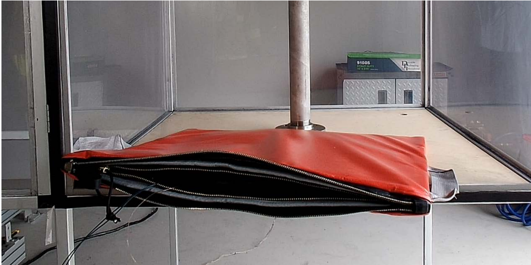
Figure 5. Laptop Inside Containment Kit
