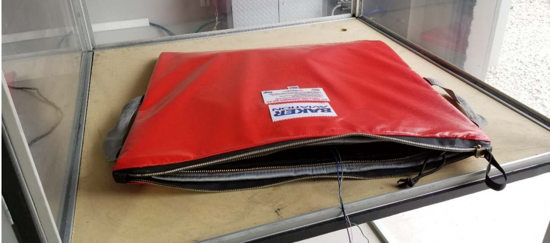
Figure 13. Laptop Inside Containment Kit
