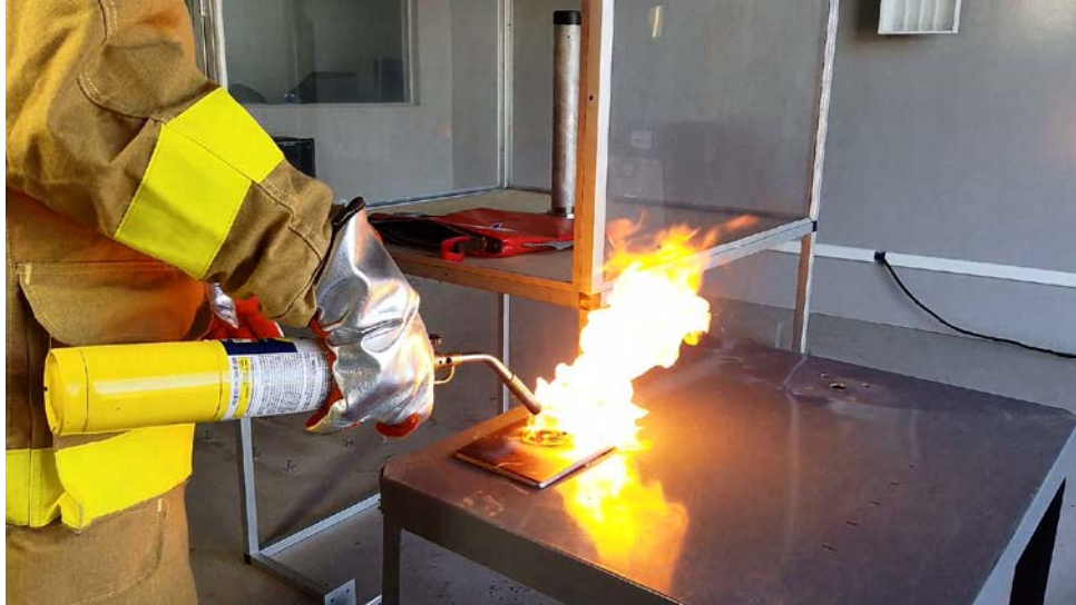
Figure 3. Propane Torch Igniting Tablet
