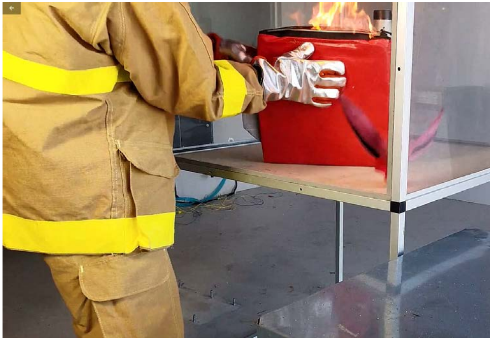
Figure 4. Tablet Dropped into Containment Kit
