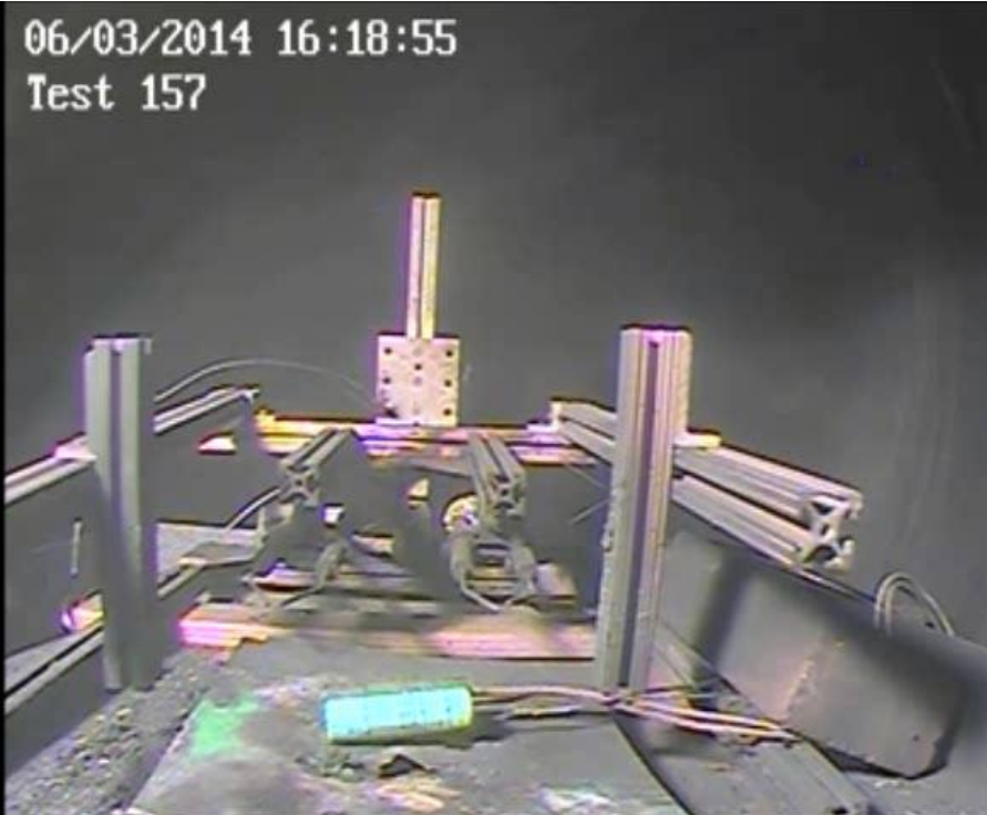
18650 Cylindrical Cell LiCoO 2 Chemistry 9.62 Whr
