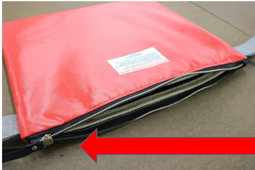
PULL TAB MISSING
